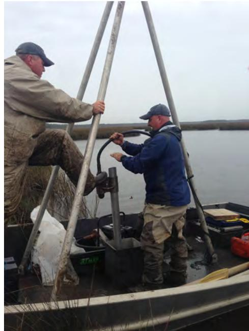
Figure 6.—Greg Taylor and Rob Tunstead demonstrate the vibracore.
